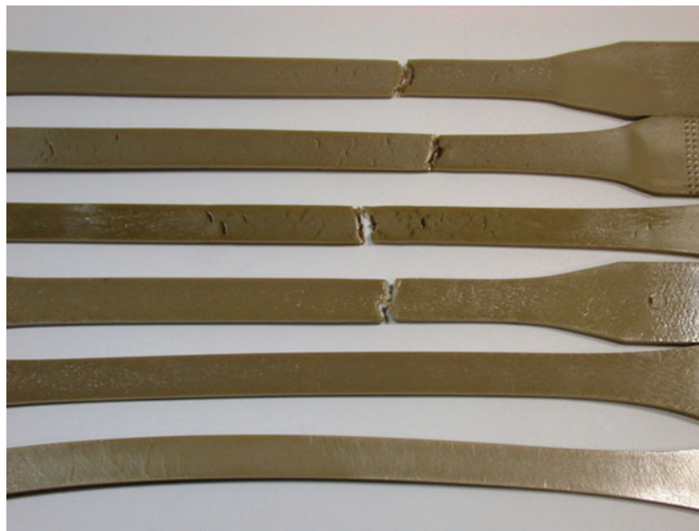
Fig. 18.16 Failed unexposed (UE) 450 G specimens tested at 121°C, 149°C and 204°C (from top down in the first three), respectively, and the failed E250, E300 and E400 exposed 450 G specimens tested at 121°C, 149°C and 204°C (from top down in the second three) respectively
