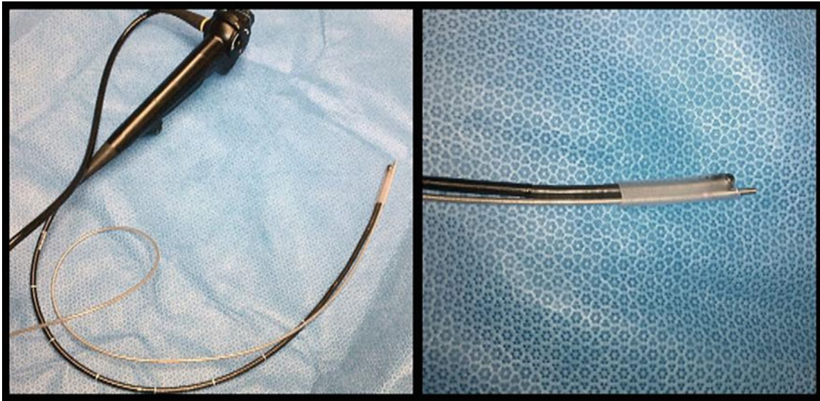
Fig. 23.8 Flexible bronchoscope with the OCT imaging probe attached to the scope exterior using a size 28 French polyvinyl-chloride nasal airway (With permission from Chest, Michel et al.)
