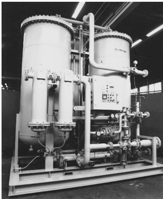
Fig. 27.4 An on-site nitrogen PSA supply system. The large vessels are absorbers and the smaller ones are dryers. (Courtesy Cirmac International, BY, Netherlands.)
