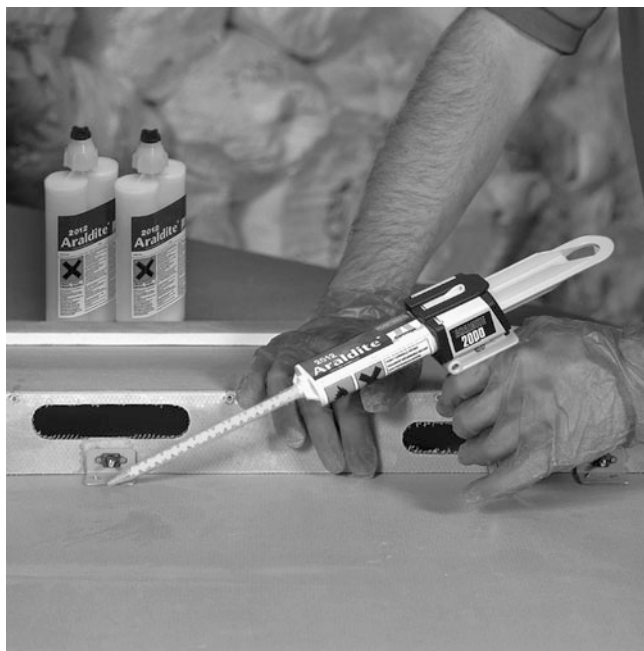
Fig. 14.4 Assembly of an aircraft headliner using an Araldite™ two-part urethane adhesive (Courtesy of Huntsman Advanced Materials)
