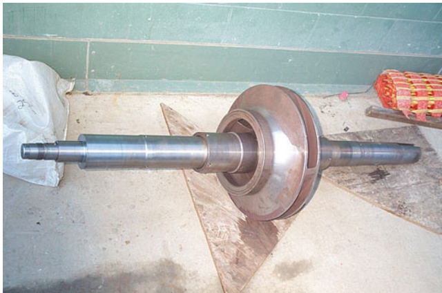
Fig. 7.5 Centrifugal pump impeller with double-sided entry (Courtesy of Millmerran Operating Company, Australia)
