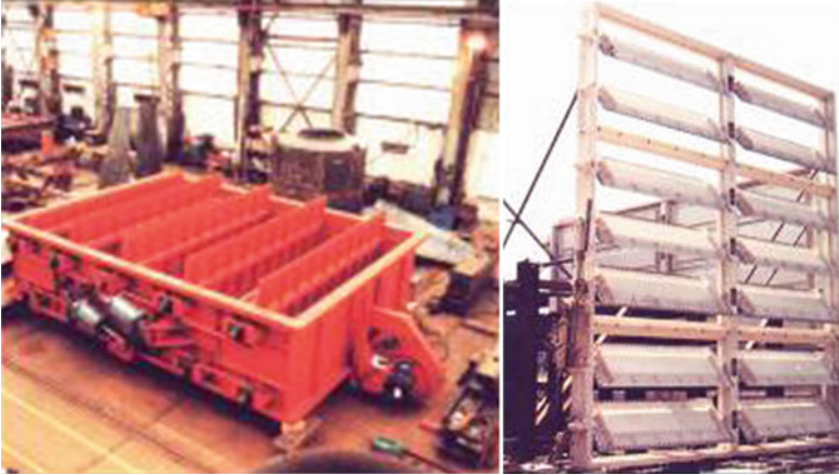
Fig. 6.2 Utility boiler louvre control dampers during manufacture (with permission of Everlee Engineering, Johannesburg, South Africa)
