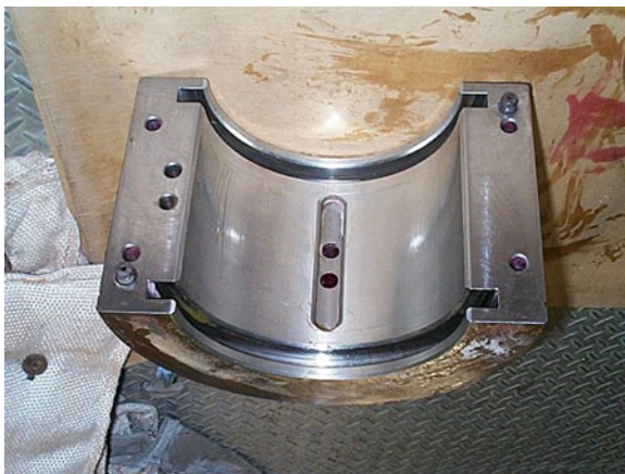
Fig. 7.16 High-pressure journal bearing showing oil entries (Courtesy of Millmerran Operating Company, Australia)
