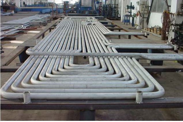
Fig. 9.6 A superheater tube platen during manufacture (Courtesy of Foster-Wheeler Corp.)
