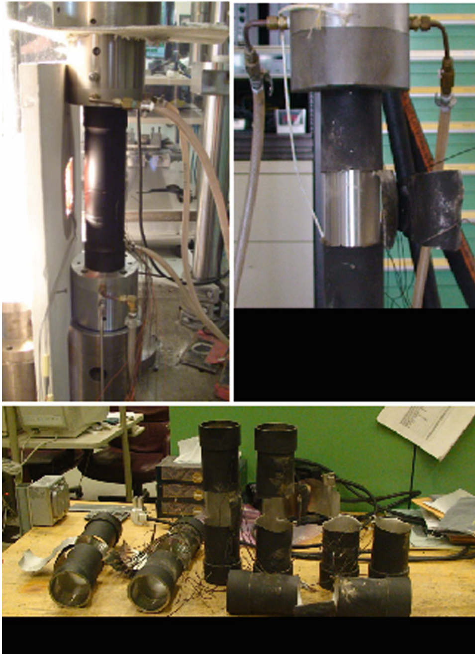
Fig. 2.7 Pressure loaded stainless steel “pipe bomb” validation experiment, resulting post-test failure and validation of repeated failure modes
