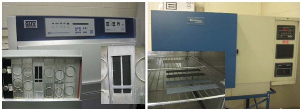
Fig. 17.1 Environmental exposure performed in the laboratory (with accelerated aging chambers) ( left , QUV/se ultraviolet radiation and condensation chamber) ( right , Tenney BTRS temperature and humidity chamber)
