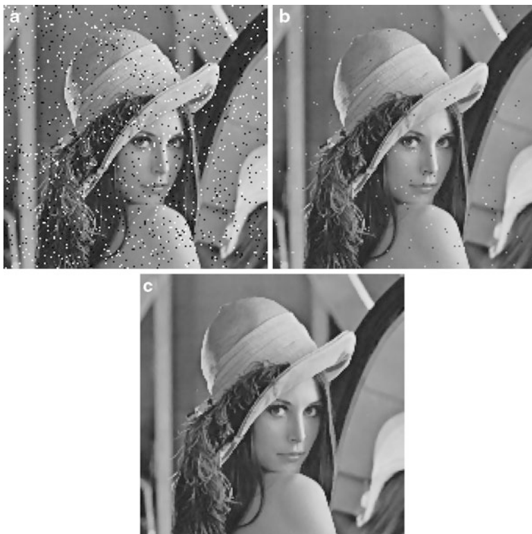
Fig. 4.16 (a) “Lena” affected by impulse noise with density 0.05, (b) denoised image (median filter of size 3 \times 3 is used), (c) denoised image ( 5 \times 5 median filter)
