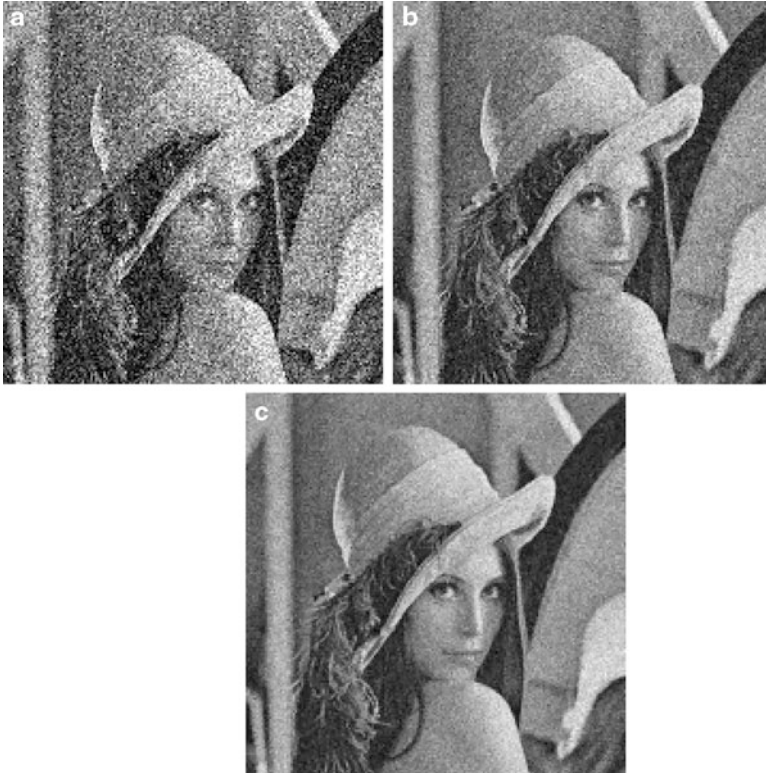
Fig. 4.13 (a) “Lena” affected by Gaussian noise with zero mean and variance 0.02, (b) filtered image obtained by using mean filter of size 3 \times 3 , (c) filtered image obtained by using mean filter of size 5 \times 5
