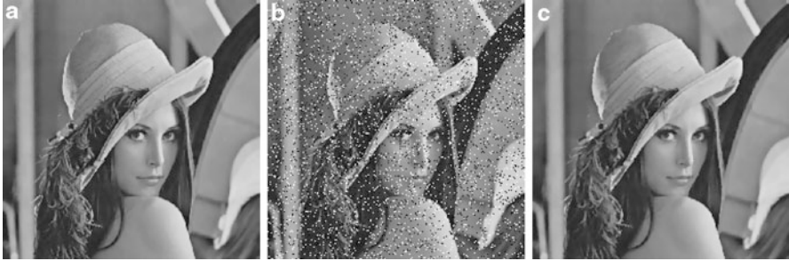
Fig. 4.46 (a) Original image, (b) noisy image, (c) filtered image
