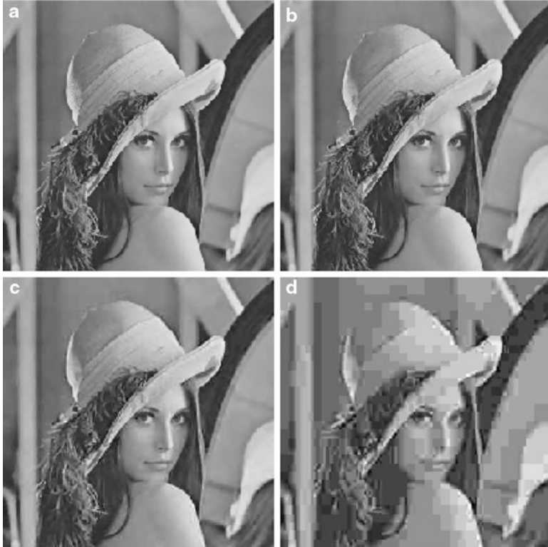
Fig. 4.25 (a) Original “Lena” image, (b) “Lena” image after applying JPEG compression with QF = 70%, (c) “Lena” image after JPEG compression with QF = 25%, (d) “Lena” image after JPEG compression with QF = 5%
