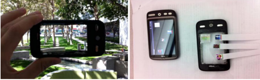
Fig. 6.2 (Left) Low-fidelity mock. The see-through hole allows users to see what is behind the device, simulating the camera. (Right) Low fidelity mock and used icons (right) next to an actual working device with the hi-fidelity prototype (left)
