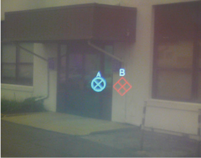
Fig. 4.2 Setting transparency of a virtual surface as a function of distance simulates the atmospheric perspective cue for the human visual system
