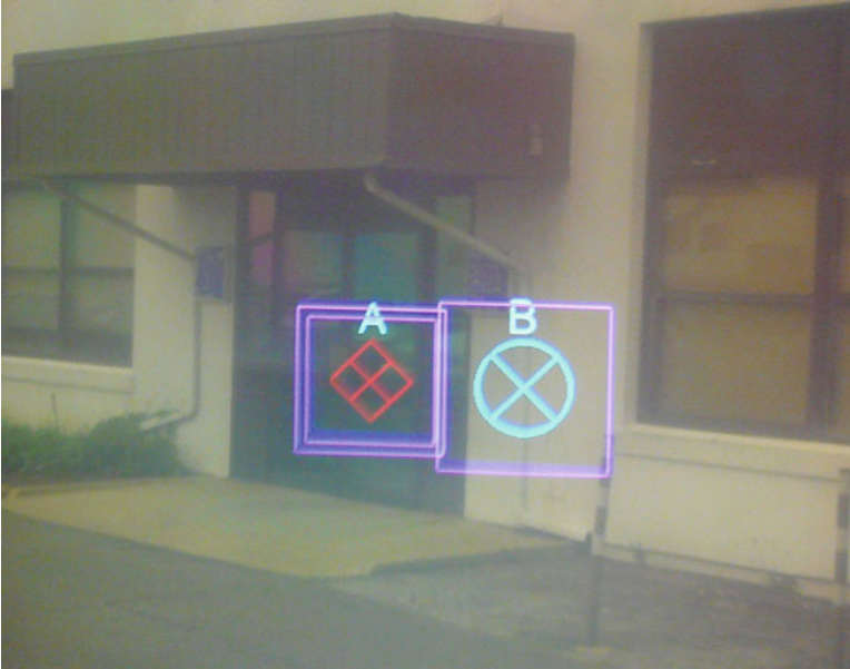
Fig. 4.11 This customized and simplified version of the virtual tunnel concentrated on the number of planes through which the tunnel was being extended to get to the target object. It was the best method in a broad-based comparison of X-ray vision metaphors [28]
