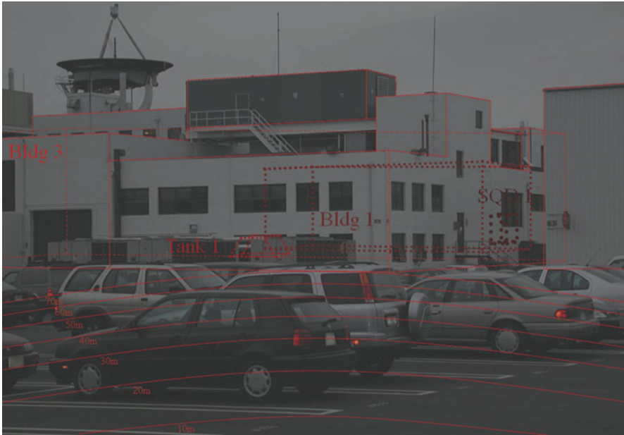
Fig. 4.6 A ground grid consisting of concentric circles can assist the user with resolving the depths of virtual and (if registration is accurate) real objects in the scene. This image is a concept sketch from 2002 and incorporates a line-based stipple technique
