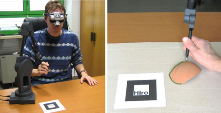
Fig. 10.6 Mechanical device-based sketching for implementing interactive AR reverse engineering modeling tool
