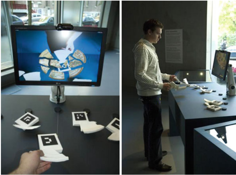
Fig. 11.3 3D printed shards create a complete virtual dish in AR on a monitor
