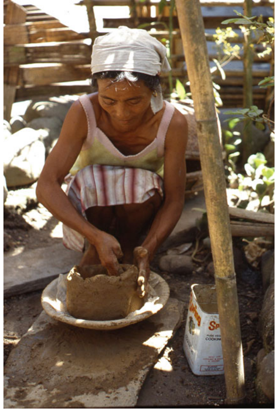
Fig. 3.12 Clay is placed on a wooden plate that is rotated during manufacture
