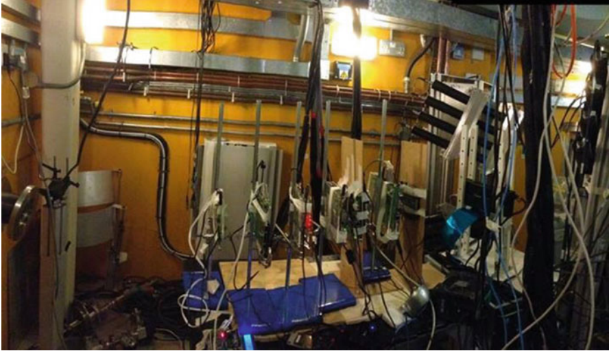
Fig. 10.14 Neutron-induced SEE in FPGAs Experiment Setup
