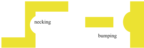
Fig. 8.10 EPE affected wires
