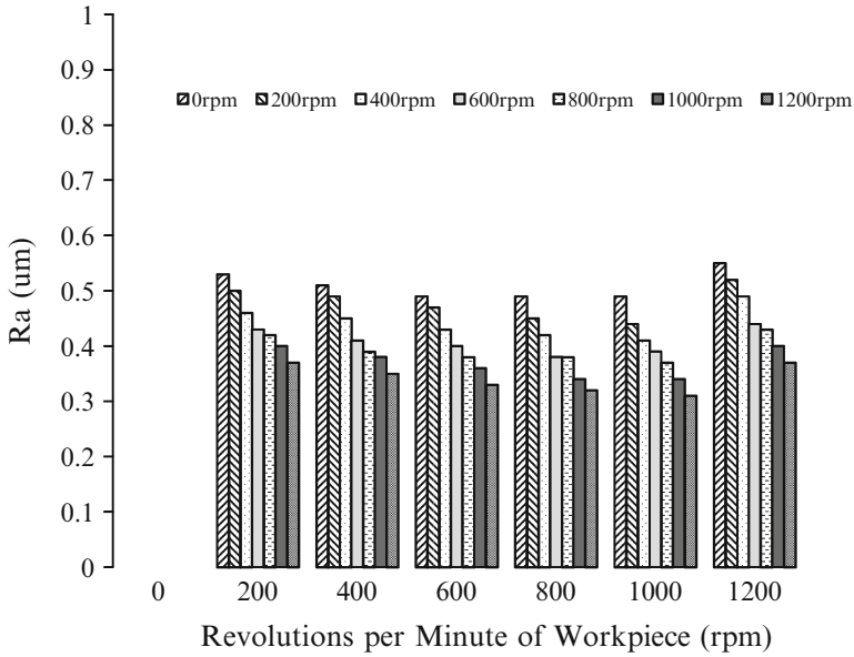
Fig. 3.149 Electropolishing at different rotational speed of electrode and workpiece (Type Ad, 4 L/min, continuous DC, 10 A, 2 mm/min, t = 3 mm, \mu = 40^\circ , R = 0.5 mm) ([71], reprinted with permission)
