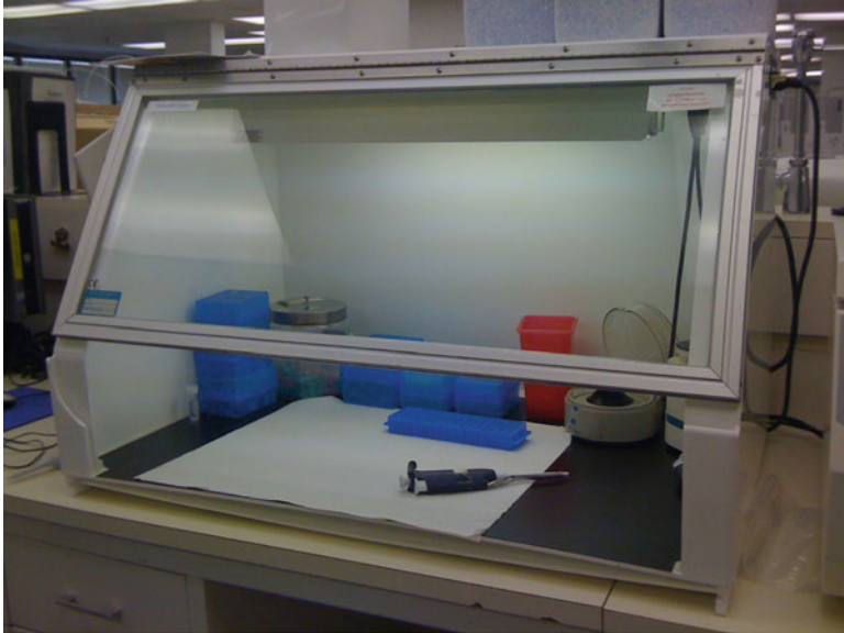
Fig. 26.2 Molecular laboratory “Dead Air Box.” The dead air box creates an atmosphere that will lower chances of contamination in molecular samples. Aerosols are blocked from entering the unit from the surrounding environment. Before and after usage, the unit can be wiped down and cleaned. Then, the unit can be closed and the UV light can be turned on to further decontaminate the area
