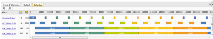
Fig. 2.5 Schedule for the SDF model of the OFDM transmitter
