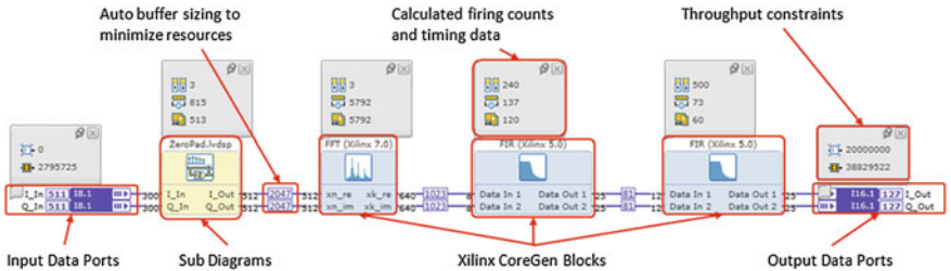
Fig. 2.4 Analysis results for the SDF model of the OFDM transmitter
