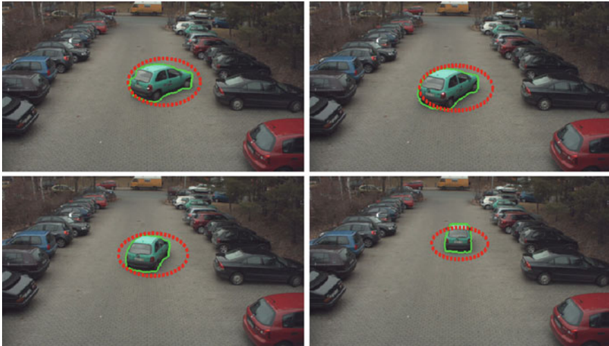
Fig. 7.6 Results of traditional mean shift tracking ( red ellipse ) compared to GMM-SAMT ( green contour ) for tracking a car on a parking lot
