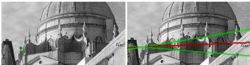
Fig. 11.3 Envelope of epipolar lines : point in the first image used for computation ( green , k^2 = 5.9915 , \alpha = 0.95 interval). Most likely epipolar line ( red ) and epipolar envelope ( green ) in the second image
