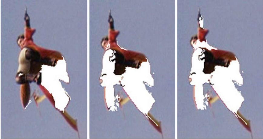
Fig. 4.5 During every iteration of the algorithm that identifies corresponding subtrees between neighboring frames new regions (marked in white ) are added to the predicted object shape in the next frame. These added regions are here shown in white . From left to right the merged object shape for the new frame after 4, 7 and 12 iterations are shown
