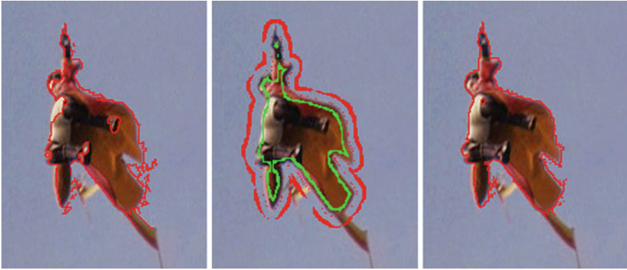
Fig. 4.7 Left initially predicted object shape (outlined in red ) which was constructed using the subtree matching approach; center automatically generated scribbles ( green for foreground, red for background); right corrected object shape, after the application of the scribbles
