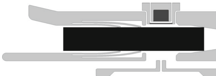
Fig. 11 Microchannel plate (MCP) hybrid-integrated in the PIMMS
