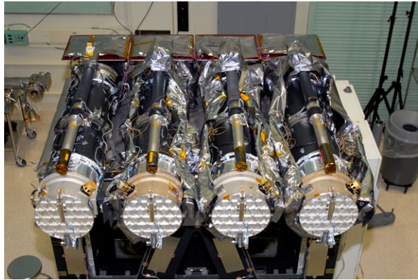
Figure 1 The AIA telescopes with their guide telescopes as seen mounted on the SDO spacecraft's instrument module during integration in the clean room at NASA's Goddard Space Flight Center.
