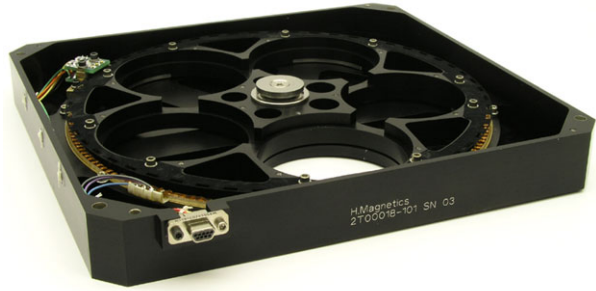
Figure 10 The AIA filter-wheel mechanism. The wheel has five openings containing various filters for each telescope as described in Table 3.
