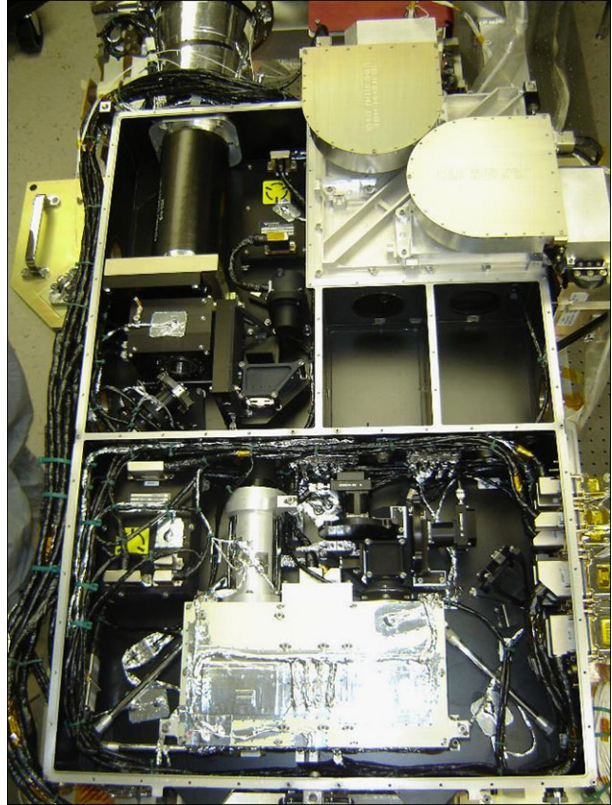
Figure 2 Photograph of the inside of the optics package. Light enters through the telescope at the upper left, passes through the chain of filters near the bottom, and is detected by the CCD cameras at the upper right. The box is roughly 88 cm long by 55 cm wide by 16 cm high. The various elements are identified in Figure 1.
