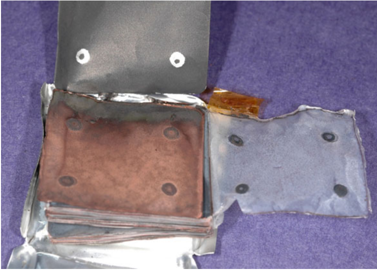
Fig. 4.9 The anode of a repeatedly over-discharged cell coated with copper
