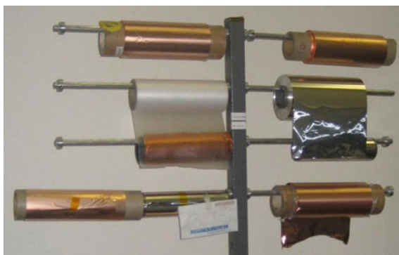
Fig. 1.14 Current collector foils prior to coating with active material
