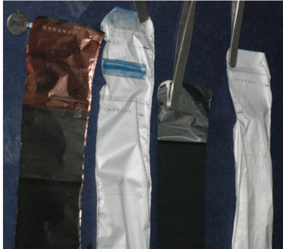
Fig. 1.15 Layers of material from a wound cylindrical cell; left to right: negative electrode (graphite coated onto copper), separator, positive electrode (metal oxide coated onto aluminum), and separator
