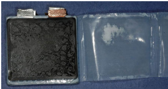
Fig. 1.2 Example of a stacked prismatic cell design
