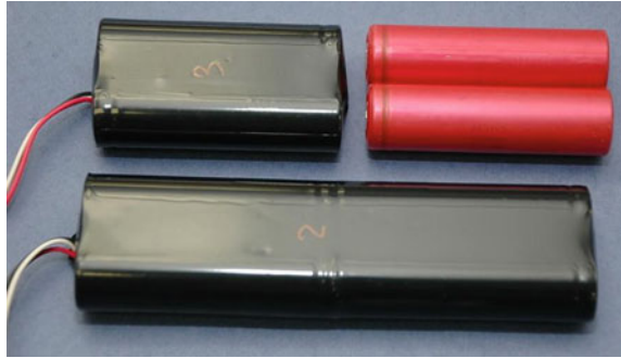
Fig. 1.19 Examples of 2- and 4-cell packs composed of 18650 cells shrink-wrapped together
