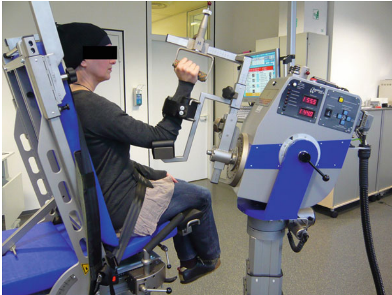
Fig. 5.6 Patient positioned on an isokinetic dynamometer (IsoMed2000, Hema, Germany) for shoulder inward/outward rotation
