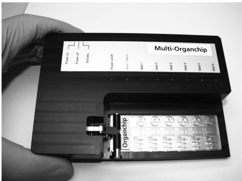
Figure 7. Photograph of a self-contained organ-on-a-chip prototype, composed of a supply unit in black and an “organ-on-a-chip” (OOC) of the standard size of a microscope slide. A holder allows for the easy and exact positioning of the OOC within the supply unit. Electrical connectors ensure the stable temperature of the OOC through sensor controlled heating at its base. Prototypes of supply units, as well as OOC devices, have been fabricated by GESIM mbH, Grosserkmannsdorf, Germany, in collaboration with F. Sonntag and coworkers at the Fraunhofer IWS, Dresden, Germany.
