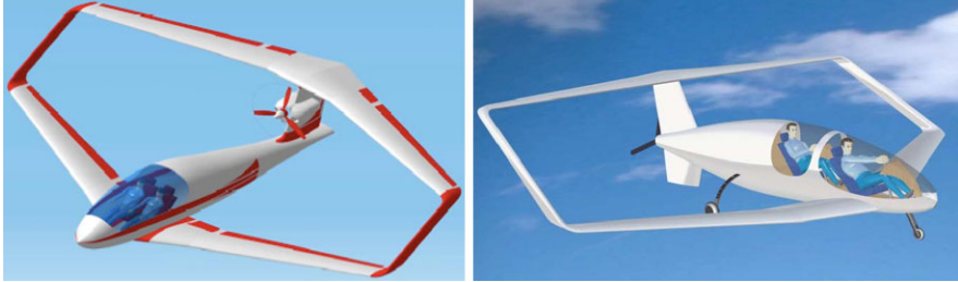
Fig. 20 Examples of ultralight PrandtlPlane
