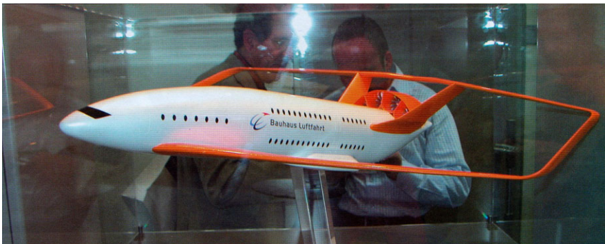
Fig. 2 Concept of a PrandtlPlane aircraft presented at the Berlin air show ILA 2008 by Bauhaus Luftfahrt
