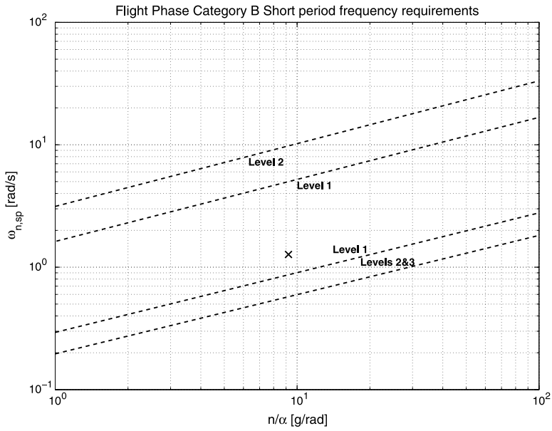
Fig. 10 Short-period frequency requirements; 150 m/s, normal cg position, sea level conditions
