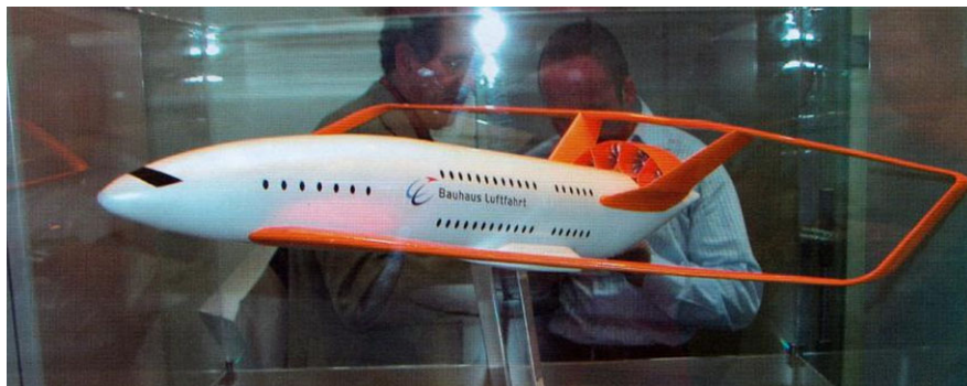
Fig. 8 PrandtlPlane configuration adopted by Bauhaus Luftfahrt
