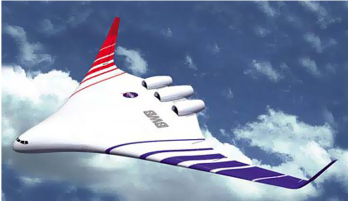
Fig. 2 Design of a Blended Wing Body by Liebeck
