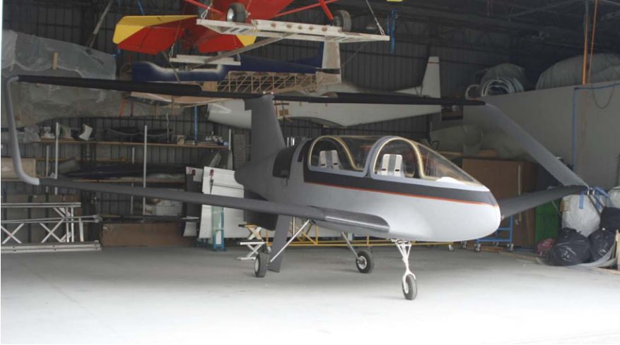
Fig. 24 Full scale prototype of an ultralight PrandtlPlane
