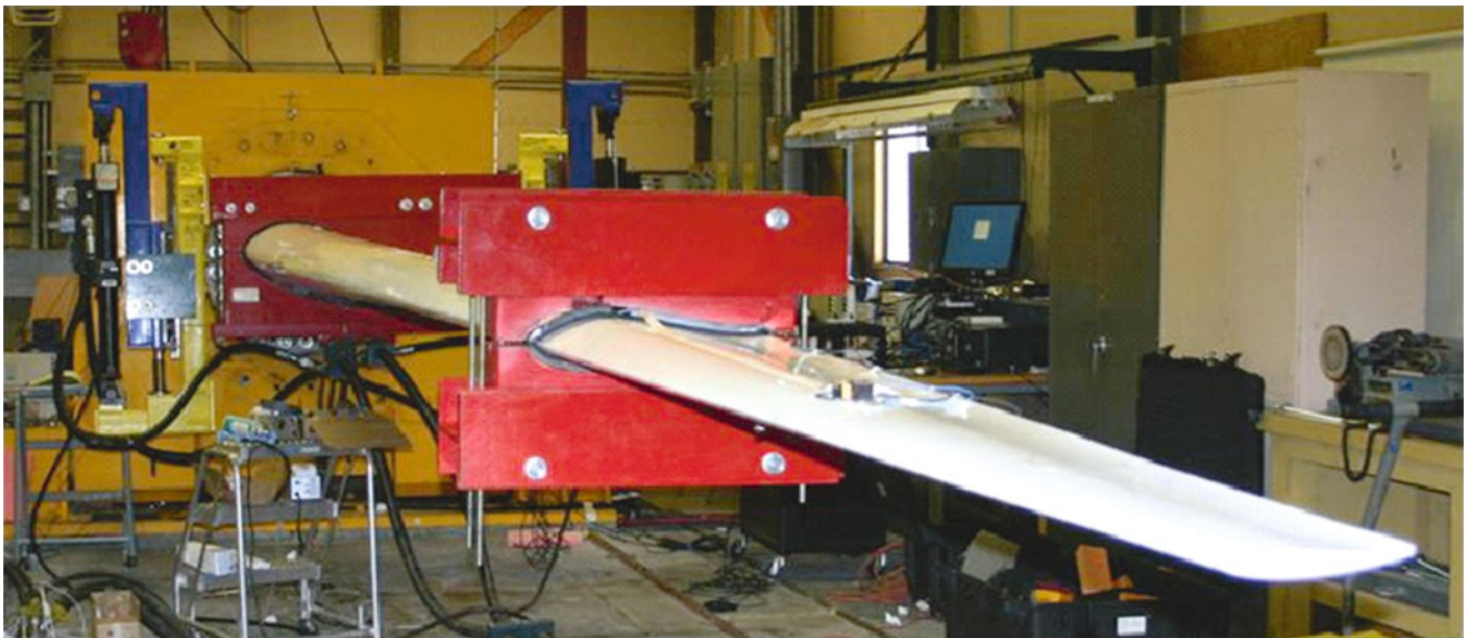
Fig. 22.12 Mass loaded CX-100, final set-up of full-scale fatigue test
