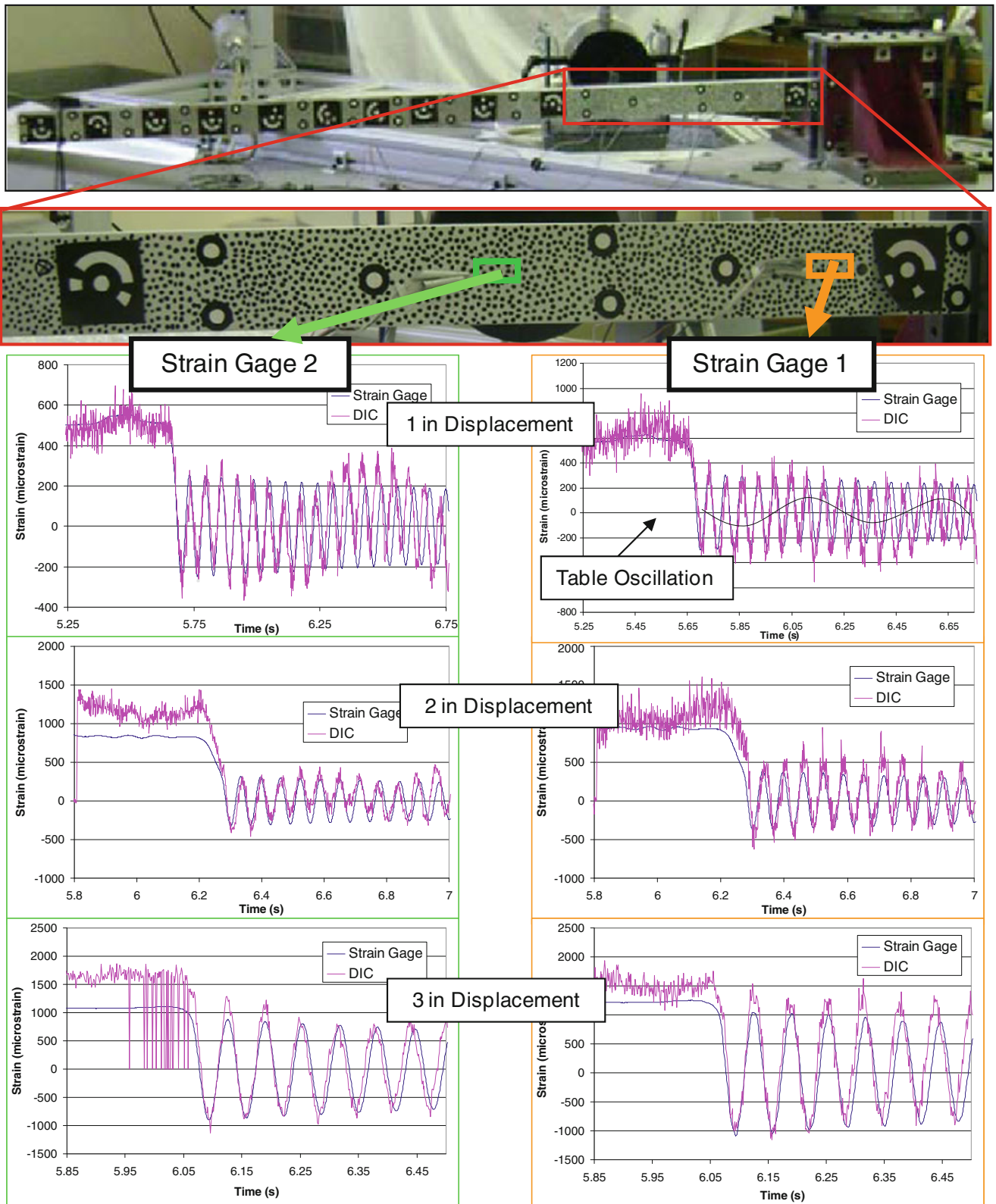
Fig. 21.2 Dynamic strain measurements from the Pluck test for three different tip displacements comparing DIC to strain gages at two beam locations
