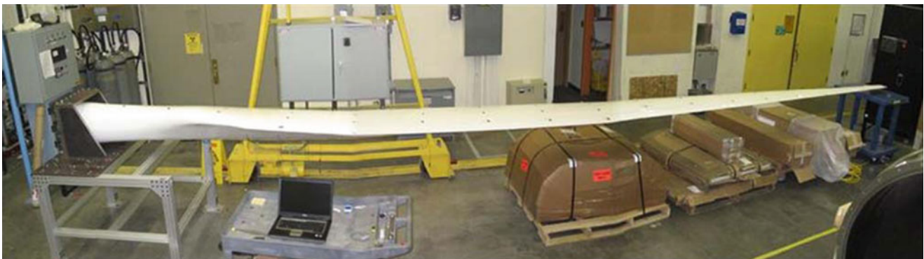
Fig. 22.6 Set-up of horizontal fixed-free modal test of CX-100
