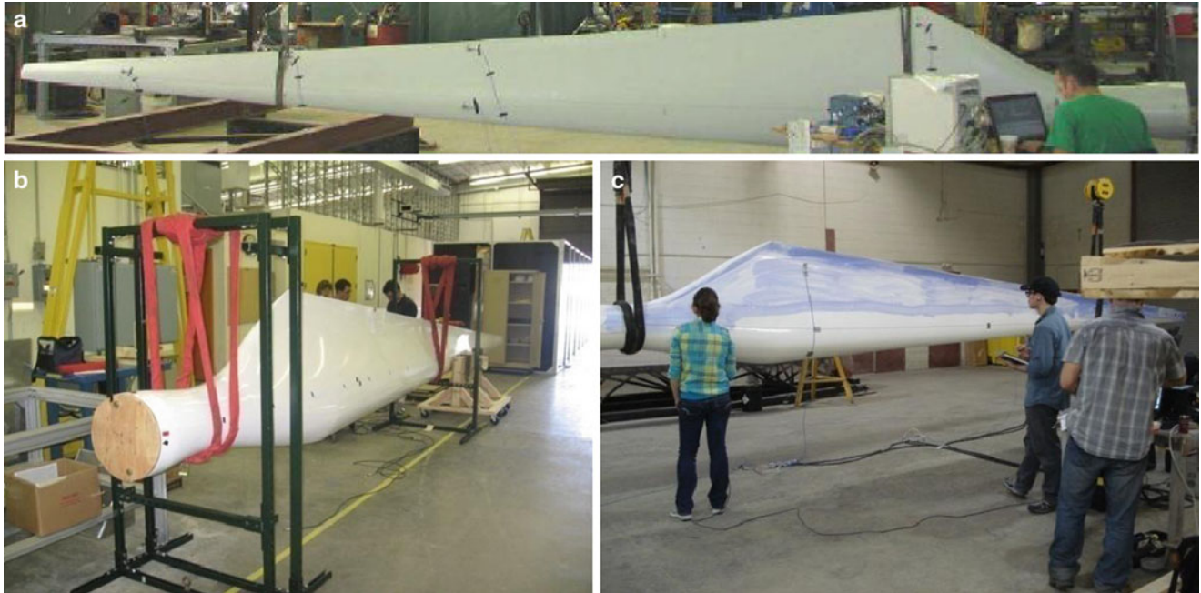
Fig. 31.2 (a) Supports used at Sandia [2]. (b) supports used at LANL [3]. (c) supports used by SDASL at TPI [6]
