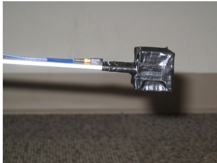
Fig. 17.4 Mass attached at tip to help drive geometrically nonlinear deformation
