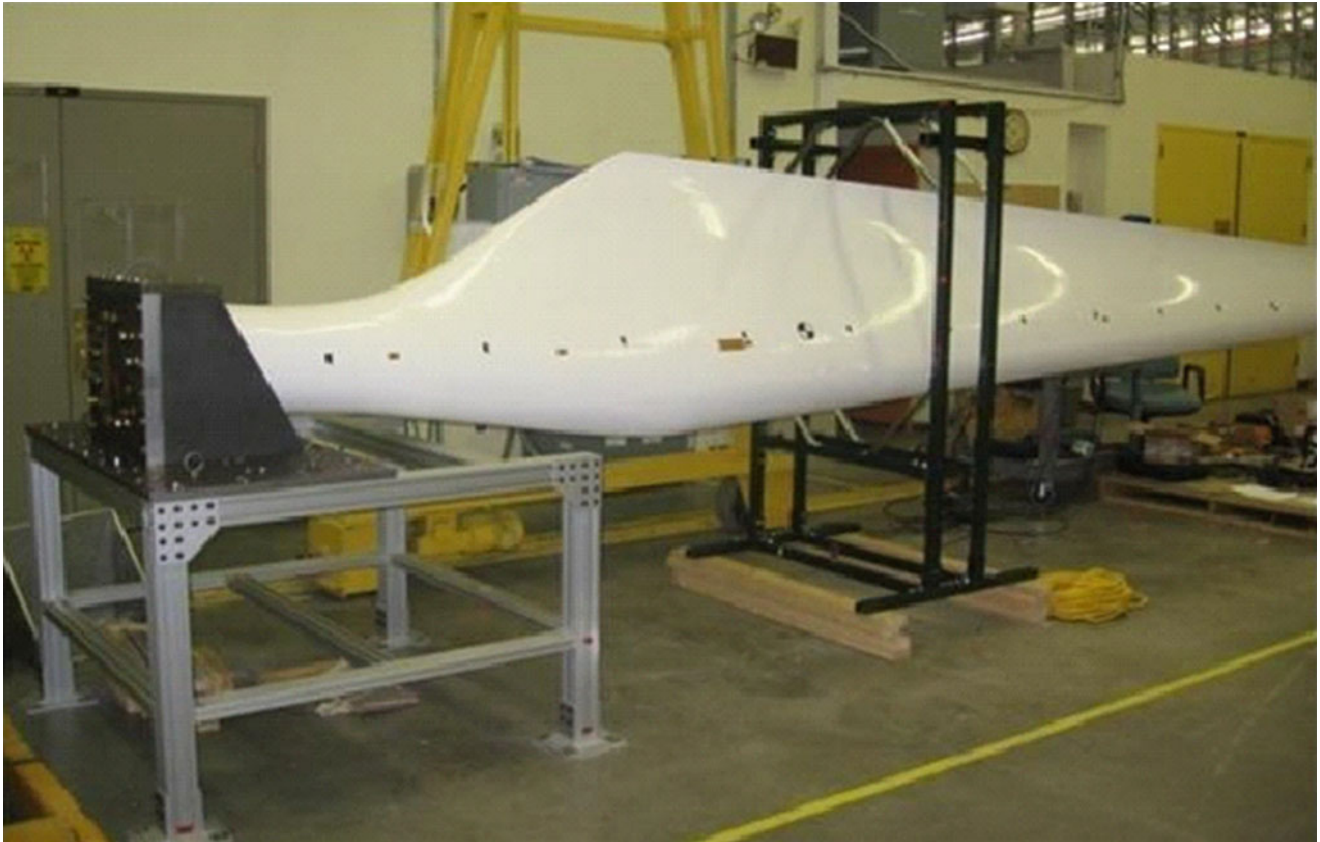
Fig. 22.2 Set-up of vertical fixed-free modal test of CX-100
