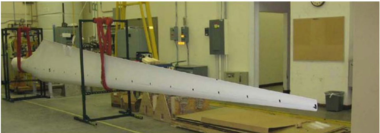
Fig. 22.1 Set-up of free-free modal test of CX-100, completed summer 2010 [8]
