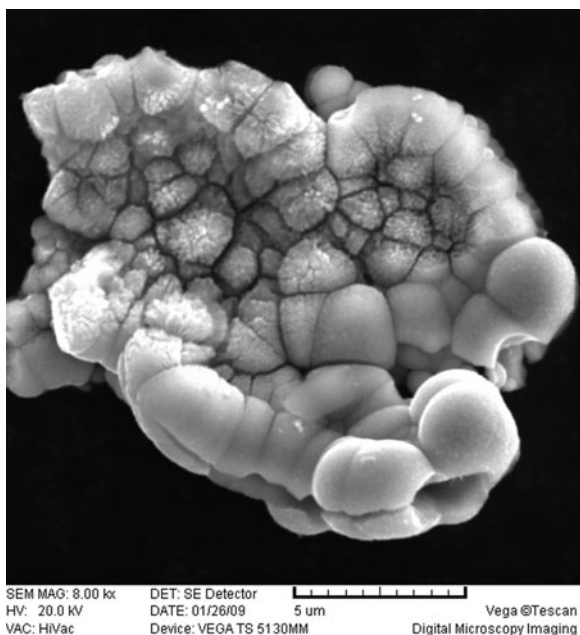
Fig. 2.46 Typical Ni powder particle electrodeposited at j_{pd}(cit) in citrate solution (Reprinted from [103] with the permission of Elsevier.)
