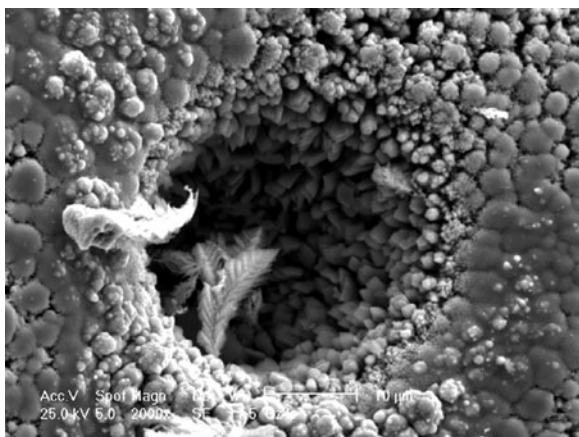
Fig. 1.21 Cobalt powder particle obtained by electrodeposition from a solution containing 1 M (\text{NH}_4)_2\text{SO}_4 , 0.7 M \text{NH}_4\text{OH} , and 0.1 M \text{CoSO}_4 at a constant current density of 0.5 \text{ A cm}^{-2} (Reprinted from [64] with permission from Springer.)
