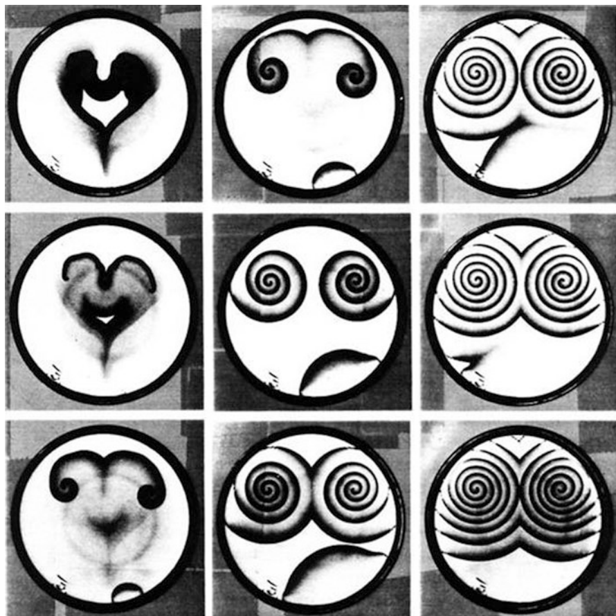
Fig. 3.1 The Belousov–Zhabotinsky (BZ) reaction. The most intensely studied chemical reaction–diffusion system (or dissipative structure) known. Reproduced from Prigogine (1980)
