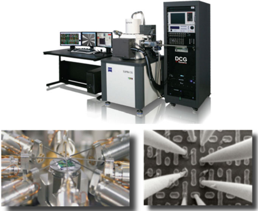
Fig. 1.4 DCG Systems' nProber Solution ( http://www.dcgsystems.com ). Eight probe nanomanipulator encoded positioners may be placed with 2nm resolution probe steps. The XYZ encoded center stage provides step and repeat capability, while allowing the probes to remain in registration while the sample is moved to the next bit (published with permission from DCG Systems, Inc., http://www.dcgsystems.com )
