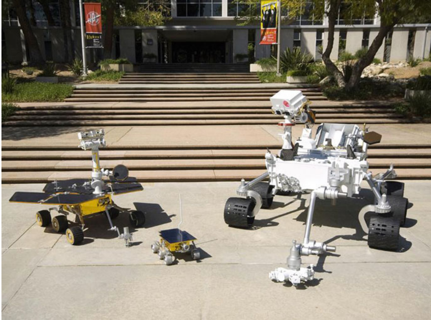
Fig. 5.1 Full-scale models of three generations of exploration rovers. Sojourner ( centre ), MER ( left ), and MSL ( right ) ( courtesy of NASA/JPL-Caltech )
