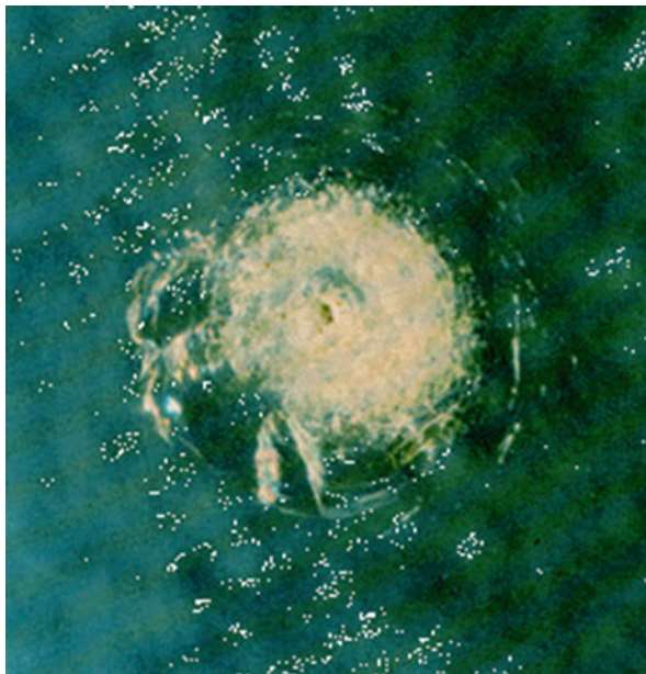
Fig. 12.3 4-mm-diameter crater on the windshield of the Space Shuttle orbiter caused by a fleck of white paint approximately 0.2 mm in diameter impacting at a relative velocity of 3–6 km/s (NASA photo)
