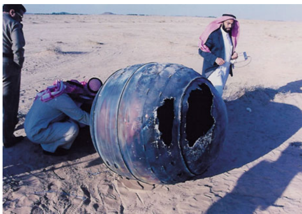
Fig. 11.4 Reentered titanium motor casting of 3rd-stage Delta 2 (Saudi Arabia, 2001) (NASA courtesy)
