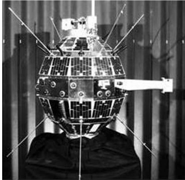
Fig. 36.2 POPPY: the first in what became the NOSS series of US maritime ELINT satellites
