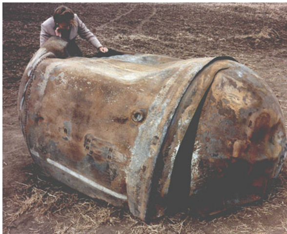
Fig. 11.3 Stainless steel propellant tank of 2nd-stage Delta 2 reentered launch vehicle (US, 1977) (NASA courtesy)
