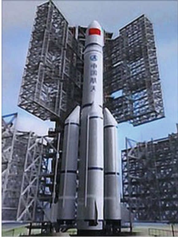
Fig. 4.2 China's powerful Long March-5 rocket in development will sport engines with the thrust of 120 t, with a test launch scheduled for 2014 (Zak 2010)
