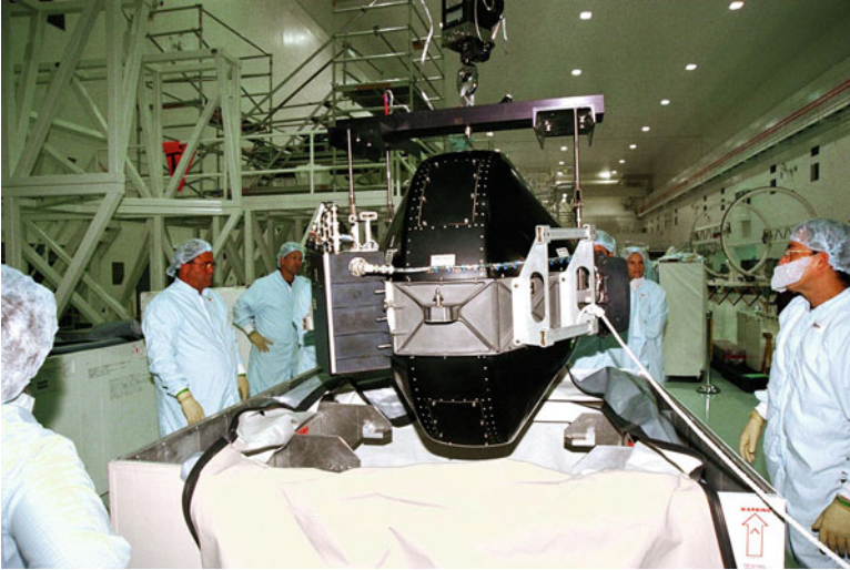
Fig. 26.4 NASA personnel handle a single control moment gyroscope for the International Space Station [12]
