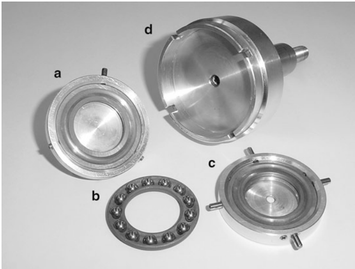
Fig. 4.32 The component parts of a single row bearing: upper casing (a), inner bearing (b), and lower casing (c) which is located in a specially modified sample support shaft (d)
