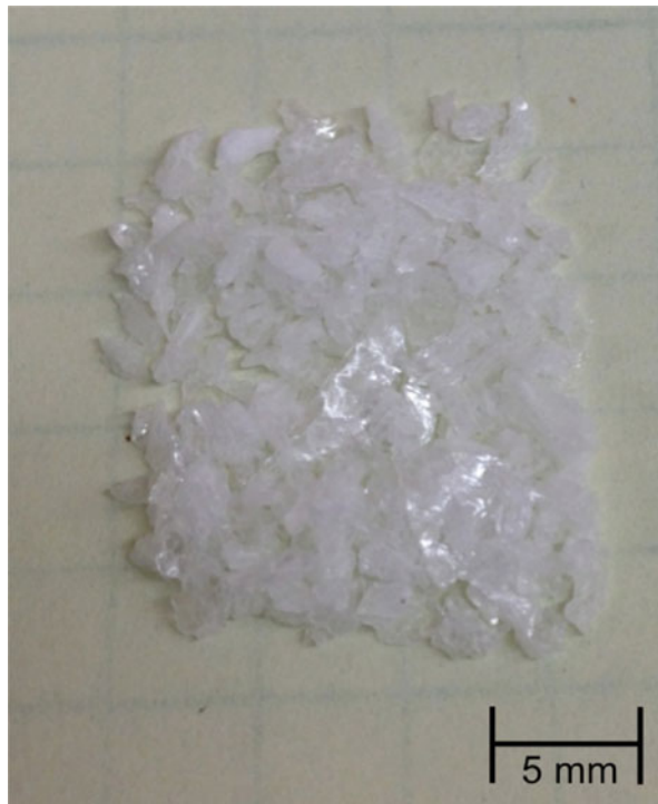
Fig. 13.6 Photograph of micron-sized boric acid ( \text{H}_3\text{BO}_3 ) powder
