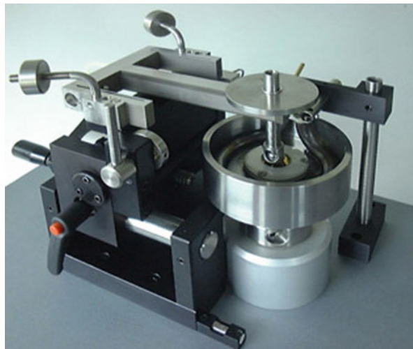
Fig. 4.17 Experimental arrangement for pin-on-disk testing of a biomaterial pair in simulated physiological saline solution. Tribological pair is submerged in a liquid cup whose contents are maintained at 37 °C by a heating coil
