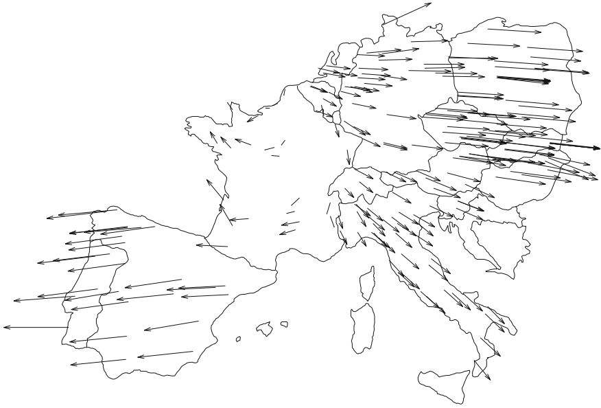
Fig. 9.4 Mode shape of the slowest electromechanical eigenvalue of a large-scale system
