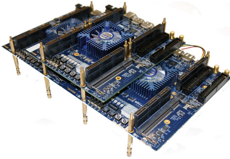
Fig. 10 1 \times 3 FPGA-array of 3 DE3 board
