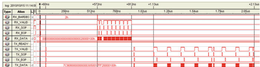
Fig. 12 Timing of the Nget and Nput schemes. The left part, between time 0 and 921, shows a data transfer from CPU memory to the NWP device (Nget). The right part, starting at time 1130, shows data transfer from NWP to CPU memory (Nput)
