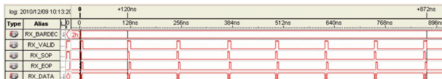
Fig. 10 Timing of the Pput implementation without write-combining. Data arrives at the NWP in portions of 16 Bytes every 120 ns
