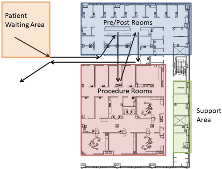
Fig. 6.2 An example of a common layout for an OPC and the patient flow process
