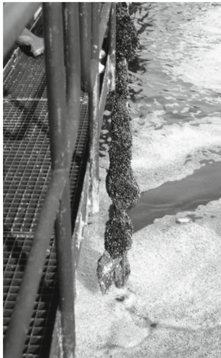
Fig. 3.2 Sampling rope exposed in seawater with first year (June–August) mussel fouling
