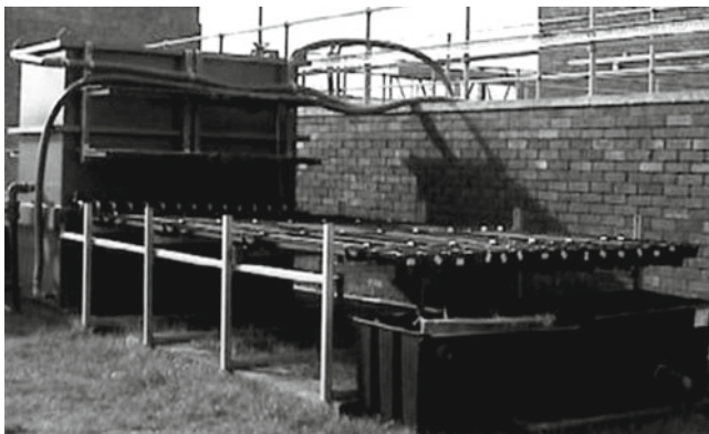
Fig. 11.8 Photograph of the experimental facility where the performance of potassium-loaded BioBullets was assessed under field conditions (Credits: Dr. Paul Elliott, University of Cambridge)
