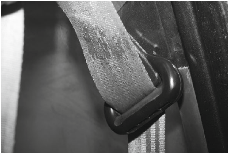
Fig. 6.9 Plastic transfer to the webbing material due to friction at the load bearing surface of the D-ring
