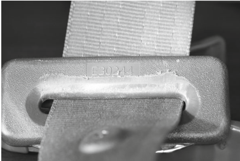
Fig. 6.8 Latch plate loading by the webbing resulting in partially melted plastic on the load bearing surface
