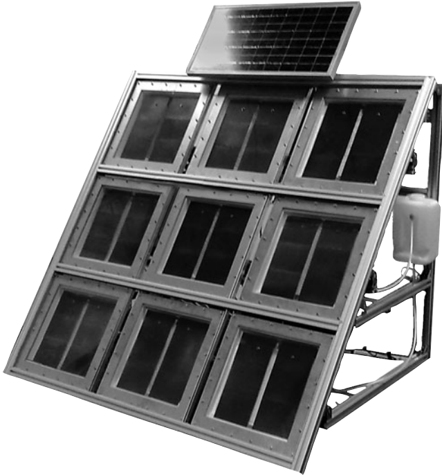
Fig. 8.1 Demonstration model of a 1-m 2 PEC array
