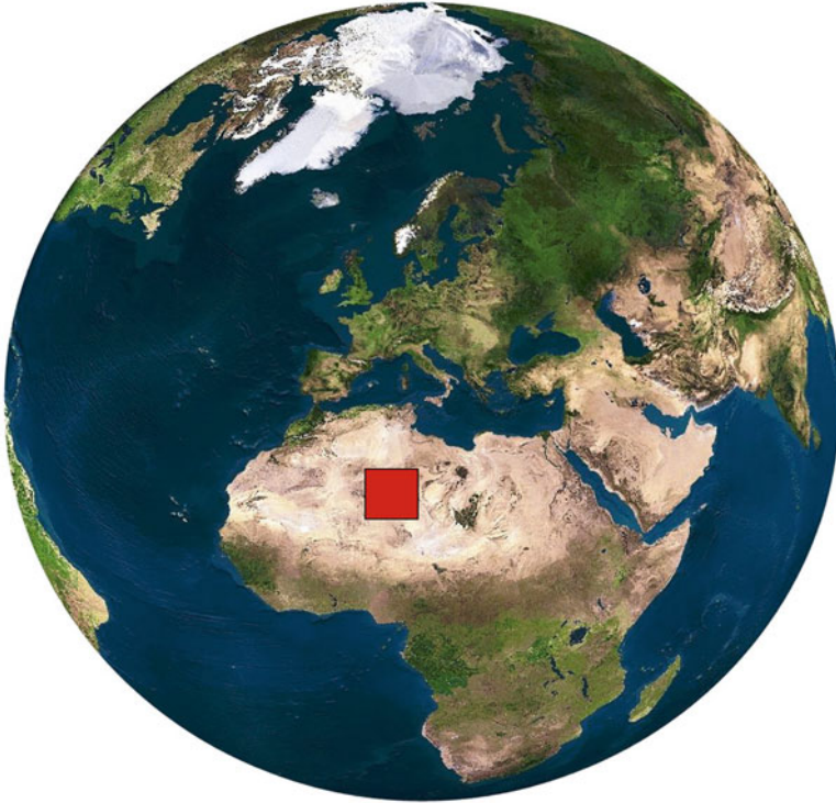
Fig. 1.1 Area of land that needs to be covered with 10% efficient solar cells in order to generate 20 TW of electrical power
