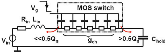
Fig. 4.10 The channel charge in a MOS device acts as a transmission line when the transistor is switched off. If the impedances on either side differ, the charge splitting is asymmetrical
