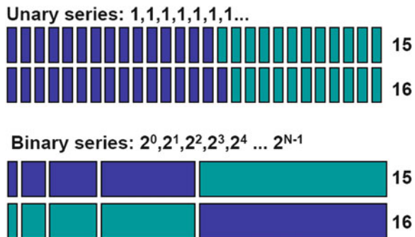
Fig. 7.1 Two basic techniques for digital–analog conversion: unary and binary representations. For both representations two signals are shown corresponding to a value of 15 and 16 LSBs
