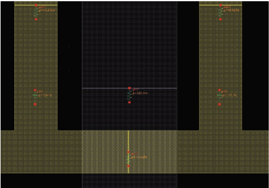
Fig. 4.16 Screenshot of parasitics in MOSFET layout having 10 fingers in TS-OPAMP layout design
