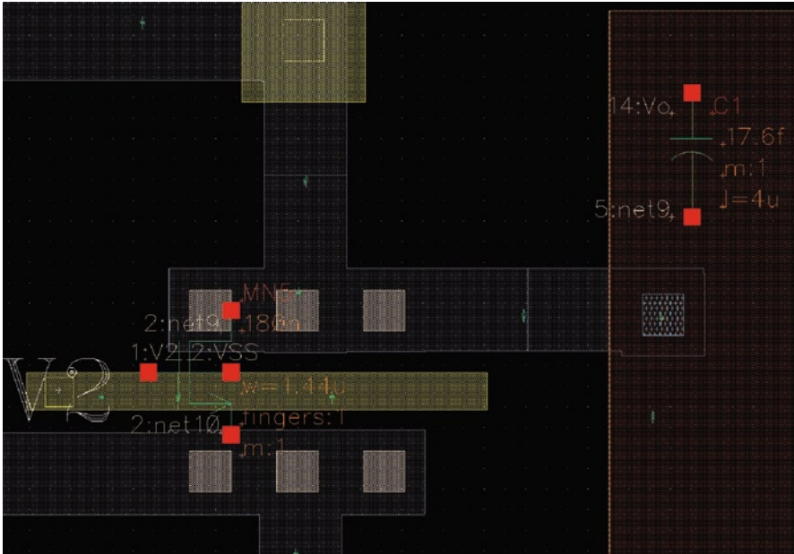
Fig. 4.17 Screenshot of parasitics identified in layout of compensation capacitor
