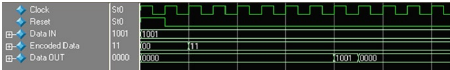
Figure 2.25 Simulation results for Viterbi decoding with two bits error in received channel data
