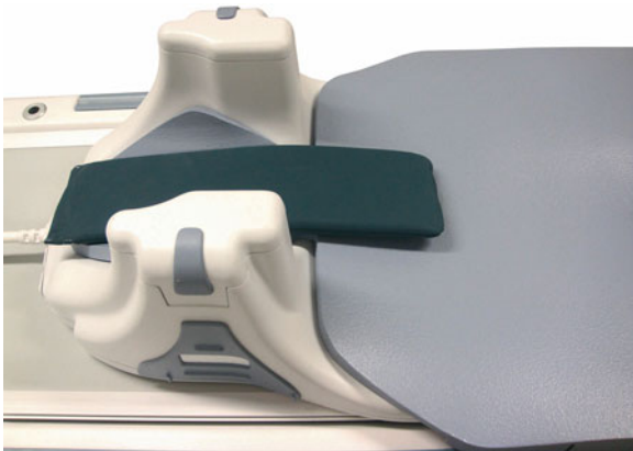
Figure 7.20 A sample dielectric pad and its proper placement on a spine coil on 3.0 T scanner.
