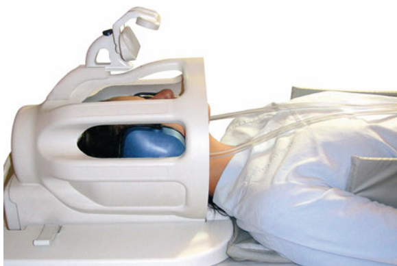
Figure 7.31 Patient positioning on an eight CH brain coil for nasopharynx or maxillofacial MRI.
