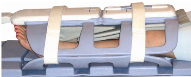
Figure 10.25 Multichannel coil can be positioned at third station if you plan to use body coil for other stations.
