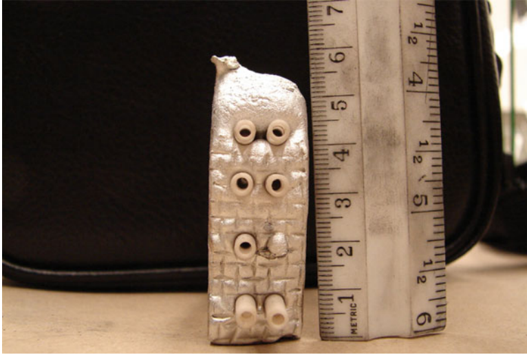
Fig. 2.9 Front view of the self-healing composite (Nosonovsky et al. 2009)
