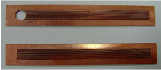
Fig. 3.45 Top view of the micro flat heat pipe (Lim et al. 2008)
