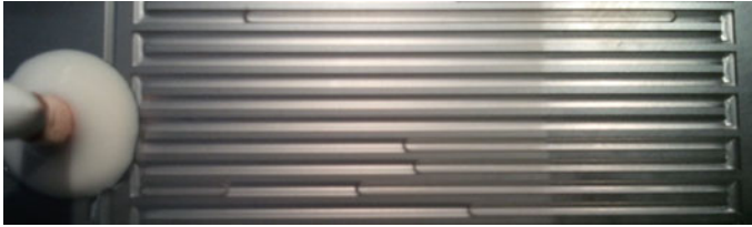
Fig. 3.42 Top view of the micro-pulsating heat pipe with filling ratio of 50 % (Youn and Kim 2012)
