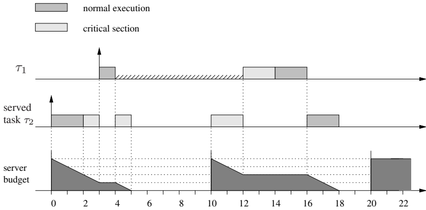
Figure 9.21 Example of extra blocking introduced when the budget is exhausted inside a critical section.
